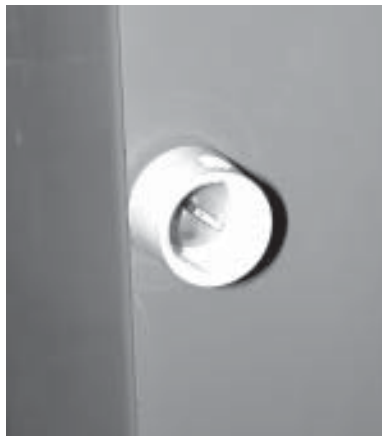
Step 2 - Slightly scratch or mar screw threads and reinstall screw inside of small cap.
