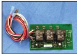
**Remedy** - add relay board HD5634 with special wiring instructions in order to take the furnace blower function away from the gas furnace control board.
