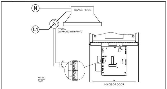
**Note:** For multi-speed vent hood installations, consideration must be made with vent hoods that include higher wattage lighting. It is possible that the low speed trigger point of the fan is equal to or lower than the current draw of the integrated lighting in the vent hood itself. In this case, the CT must be installed at the motor in the vent hood minus the lighting.
