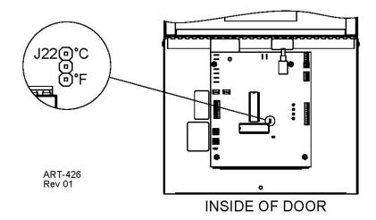
**NOTE:** Factory default is °F. A power down reset is required upon changing of this jumper.
