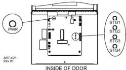
**Red LEDs** – there are 4 red LEDs on the control, each LED represents a stage of electric heating elements. This chart shows watts per red stage LED based on model number.
