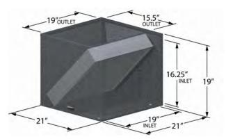
Standard 1" filter (20" x 20") – field installer could arrive at filter filler bracket for slip-in within the provided rails.
